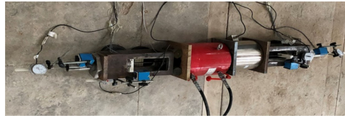
Figure 6. Pullout test device for the composite anchorage.
