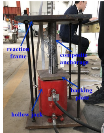
Figure 5. Pre-tightening equipment for the composite anchorage.
