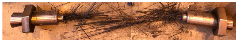
Figure 22. Failure mode of anchorage CER-5.
