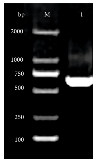
FIGURE 1: Agarose gel electrophoresis of hpaA gene fragment amplified by PCR from H. pylori . Lane M; DNA marker; lane 1: amplified hpaA gene (648 bp).
