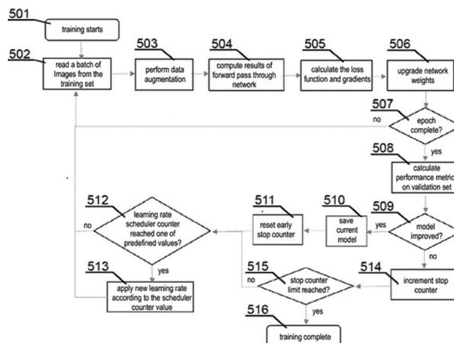
**Figure 1:** An outline of the machine learning process used to train the neural network which placed pedicle screws on the computed tomography radiographs
