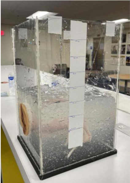
Figure 2 Synthetic vaginal model in a sealed acrylic case (A) with the addition of gel to simulate intravaginal pressures (B).
