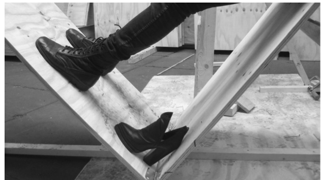
Fig. 2 Experimentation to discover unconventional affordances for supported standing. Slanted support for feet is experienced as comfortable when combined with a scaffolded leaning position. When seeking a right angle for the planks that support parts of the body (e.g., feet and upper body), people's experiences of better and worse angles typically have an affective component. For example, when support for their feet is too flat they will often experience dissatisfaction whereas foot supports that form 90° angles with the planks that support their upper body typically give an optimal grip, feel much better and reduce this discontent (see also the discussion of discontent experienced by architects presented in an earlier work [10]). Photograph reproduced with permission from Rietveld Architecture-Art-Affordances
