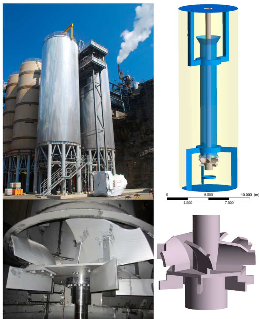
Figure 1. Industrial scale OKTOP@9000 reactor (left) (Outotec Plc., n.d. 22 ) and CAD geometry for large-scale reactor and impeller (right). Credit line: Adapted with permission from http://www.outotec.com/products/leaching-and-solution-purification/zinc-concentrate-direct-leaching . Copyright Outotec Oyj 2018.
