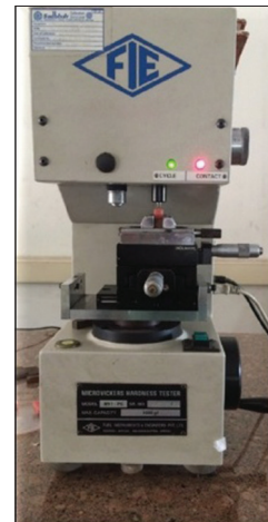
Figure 4: Surface microhardness measured using digital Vickers microhardness tester
