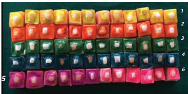
Figure 3: Acrylic blocks with different nail varnish application for each group
