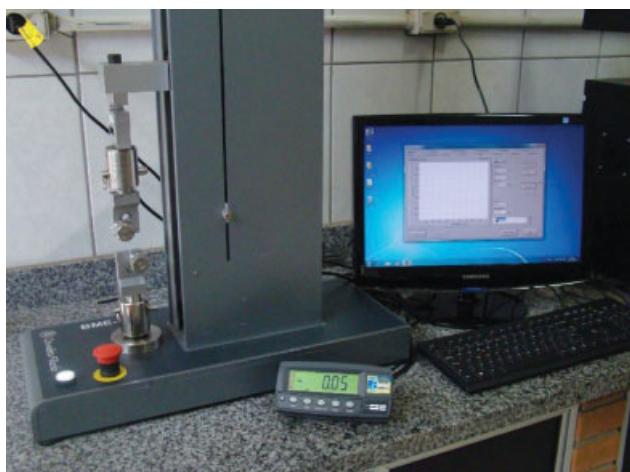
Fig. 2 Experimental equipment for tensile assays: BME 10 kN test machine, 50 kgf loading cells and fixation claws.
