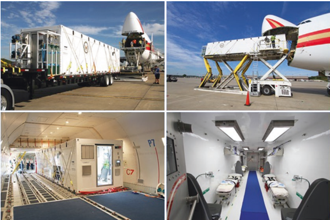
Fig. 20.3 The Containerized Biocontainment System (CBCS) was developed to transport up to four patients with highly infectious diseases on a modified 747 or mili-
