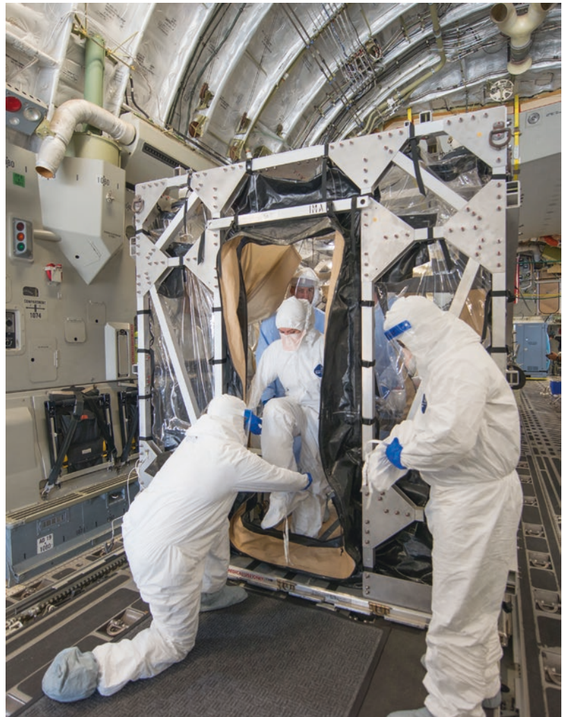
Fig. 20.4 The USAF Transportation Isolation System (TIS) is a modular system that can transport up to eight patients with highly infectious diseases. AE crew members wearing personal protective equipment are exiting the TIS during Exercise Mobility Solace at Joint Base Andrews, Maryland (US Air Force Photo/Airman Megan Munoz)
