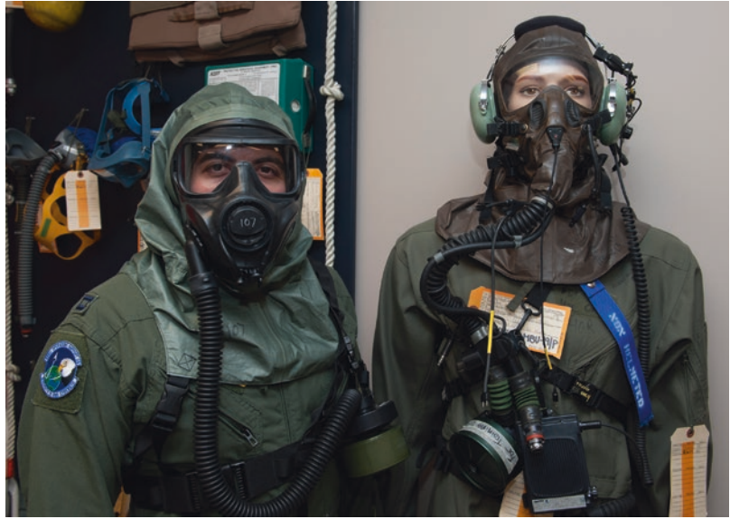
Fig. 20.5 An aircrew member wears the XM69 Aircrew Chemical, Biological, Radiological, and Nuclear (CBRN) Defense system while standing next to a mannequin wearing the legacy US Air Force Aircrew Eye/Respiratory Protection (AERP). (US Air Force photo/Senior Airman Zachary Cacia)
