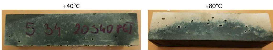
Figure 2. Specimens with 20% activator cured at 40 °C or 80 °C for 12 h.
