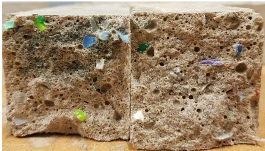
Figure 7. Cross sections of specimens (from left: mortars 10S80P and 10S40P).
