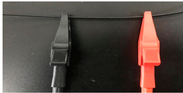
Figure 3. Measurement of the resistance of conductive ABS filaments.
