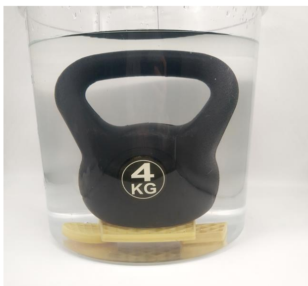
Figure S33. Under water weight loading test of 3D printed model.
