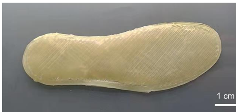
Figure S39. 3D printing insole with LiNTf 2 (5 wt%).
