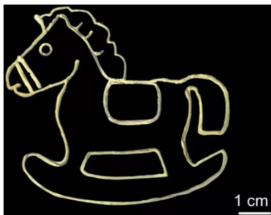
Figure S29. 3D printing pattern of poly(TA) by 3D printing pen.
