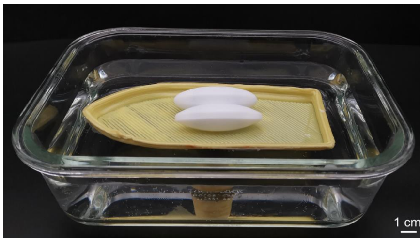
Figure S35. 3D printed boat on water loading 42.6 g.
