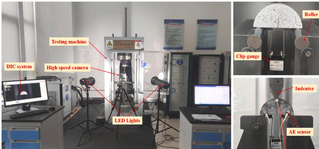
Fig. 2. The experimental setup and measuring methods.
