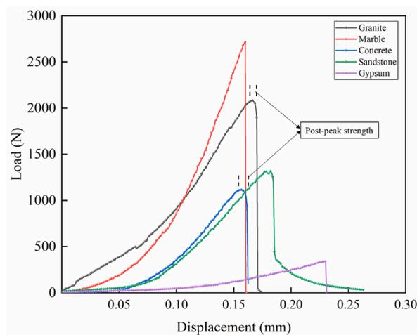
Fig. 4. The load-displacement curves of all specimens.
