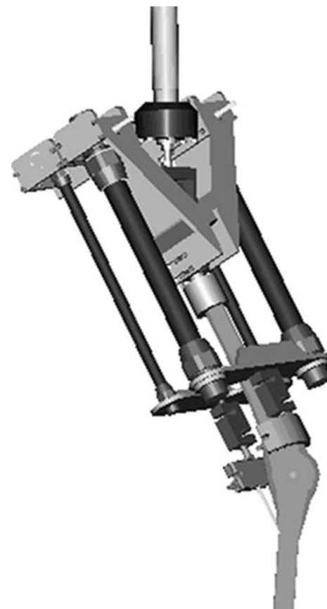
Fig. 1 Schematic drawing of the knee simulator that was used for this study
