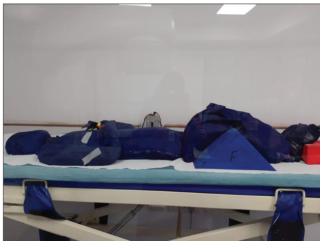
Figure 2: Shows the photograph of rice flour phantom in supine position on the treatment couch with bent knees
