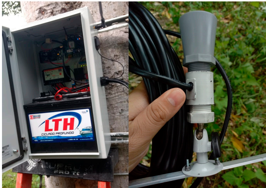
Figure 19. Electronic boards and ultrasonic sensor.
