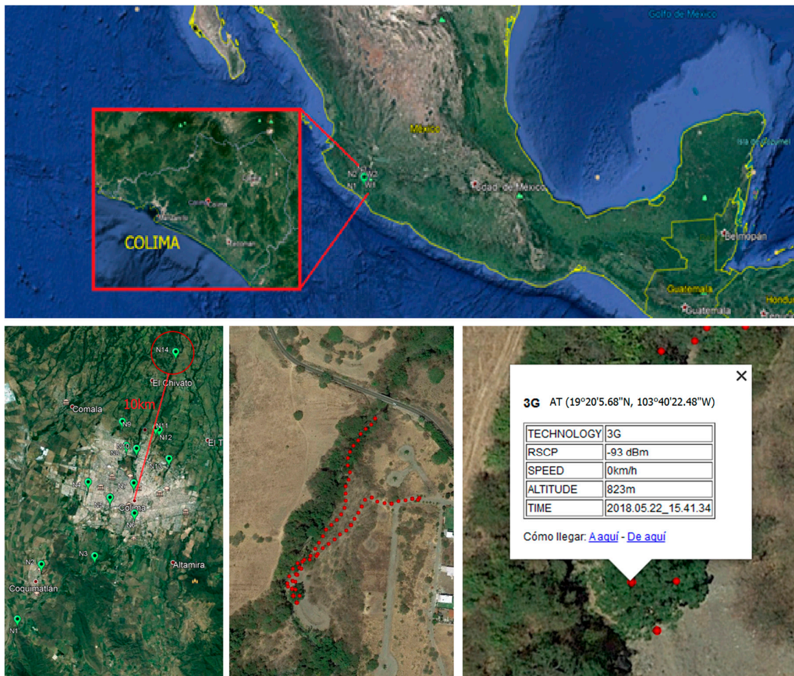
Figure 16. Field work: 3G signal measurements for deployment.
