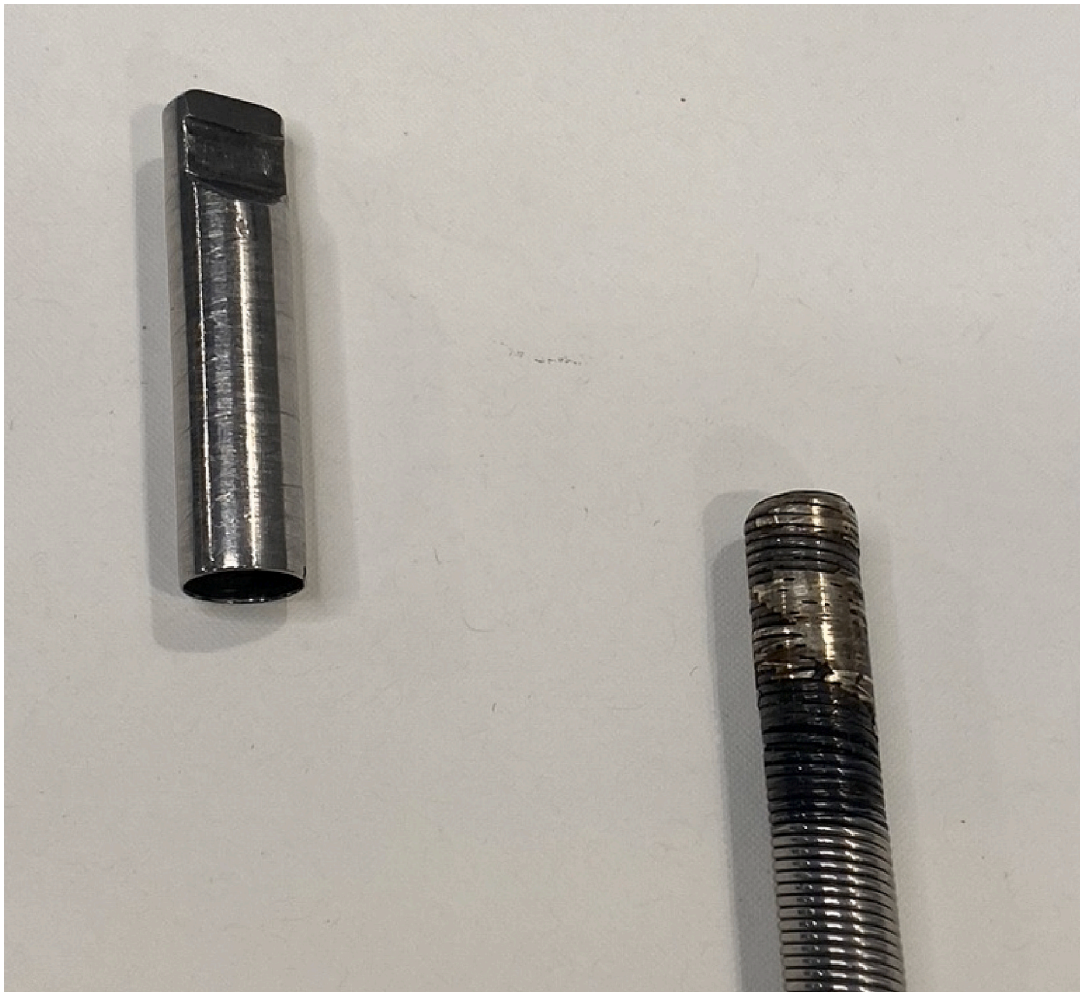
Fig. 2. Picture of intramedullary reamer showing dissociation of the reamer head from the shaft. Note burnishing of the reamer shaft.
