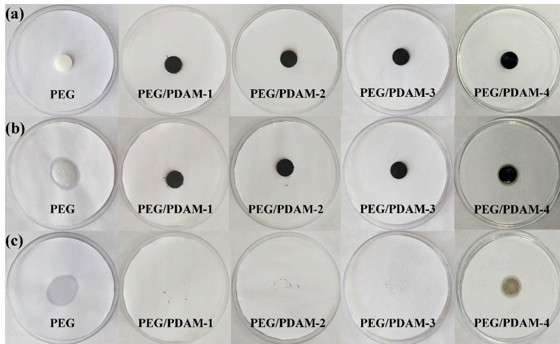
Figure 4. Leakage test photographs of PEG, PEG/PDAM-1, PEG/PDAM-2, PEG/PDAM-3, and PEG/PDAM-4: (a) pictures of samples before the thermal stability test; (b) pictures of samples after the thermal stability test; (c) pictures of leakage trace after the removal of samples.
