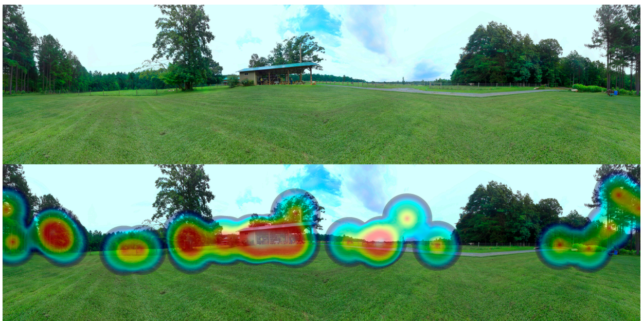
Figure 3. Example of an unfolded virtual environment without ( above ) and with ( below ) a heat map visualization of points generated with the place marker application.
