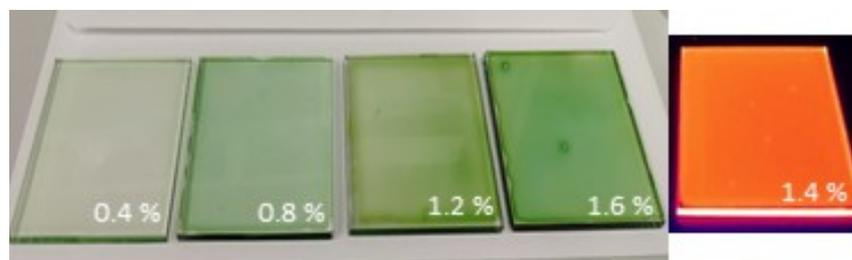
**Figure 7.** Examples of  $50 \times 50 \times 3$  mm<sup>3</sup> LSC devices containing compound **1c** at different concentrations (left), as well as LR305 at 1.4 wt% (right).
