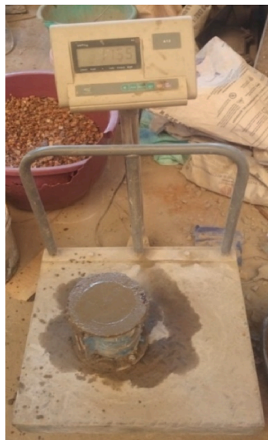
Fig. 5. A fresh concrete sample being used to measure fresh density.
