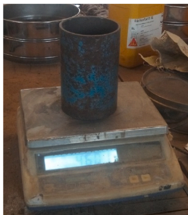
Fig. 2. Weighing a cylinder for density test.
