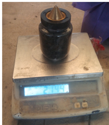
Fig. 3. A sample of a filled pycnometer being weighed.
