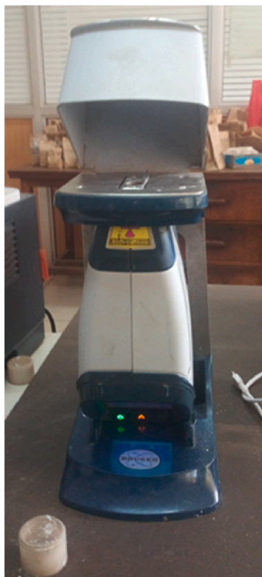
Fig. 1. An XRF gun for the analysis of chemical composition.
