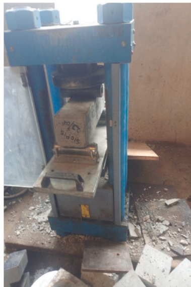
Fig. 8. An example of a sample experiencing the flexural strength test.
