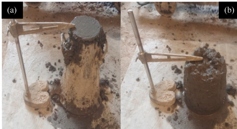
Fig. 4. A sample of the slump test that was done on the concrete mixes. (a) before the removal of the slump cone (b) following the removal of the slump cone (ii) Fresh Density.
