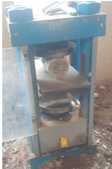
Fig. 7. An example of a sample experiencing a split tensile strength test.
