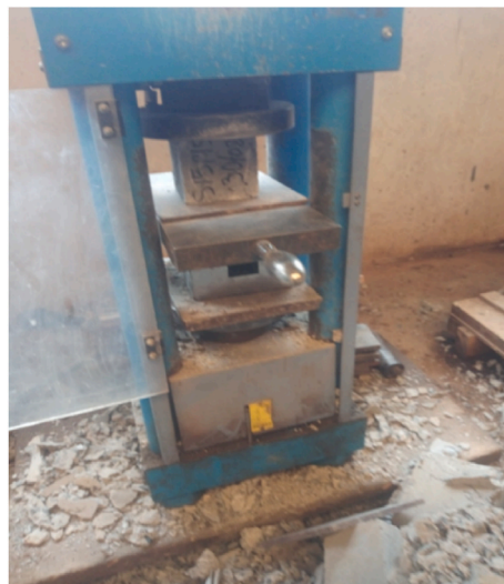
Fig. 6. An example of a sample experiencing compressive strength test.
