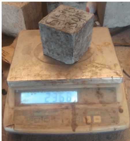
Fig. 9. A cubic specimen sample that is being weighed using a balance.
