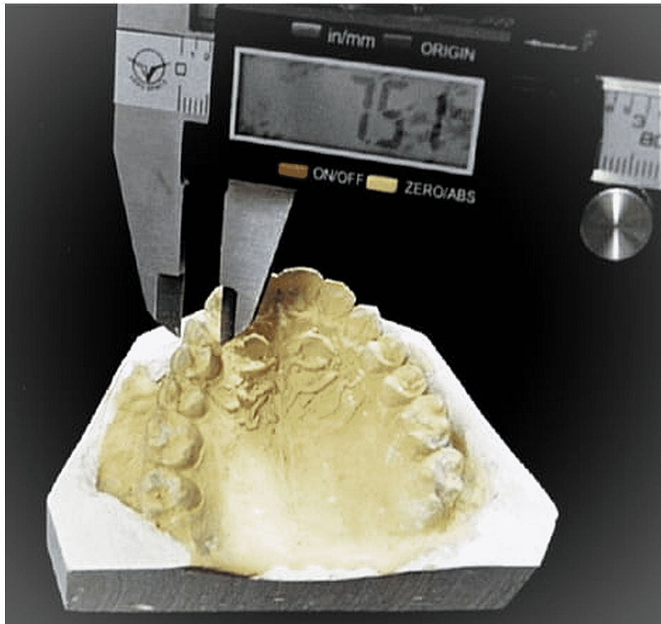
FIGURE 2: Vernier caliper measurements on the cast
