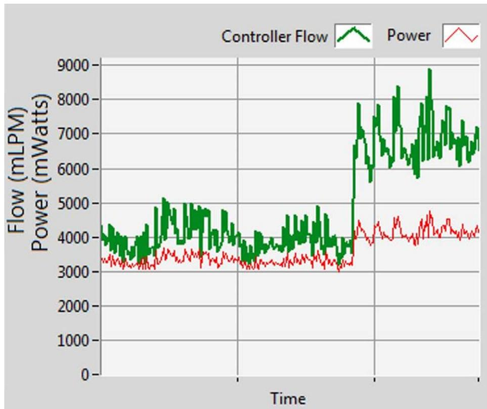
**Figure 3.** Thrombus ingestion power signature as demonstrated by sudden elevated pump power and calculated flow.
