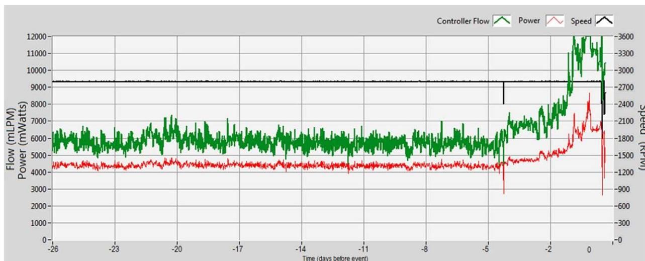
**Figure 1.** Power and calculated flow increase as a result of pump thrombus observable in logfile data (red = average power, green = average flow, black = pump speed).
