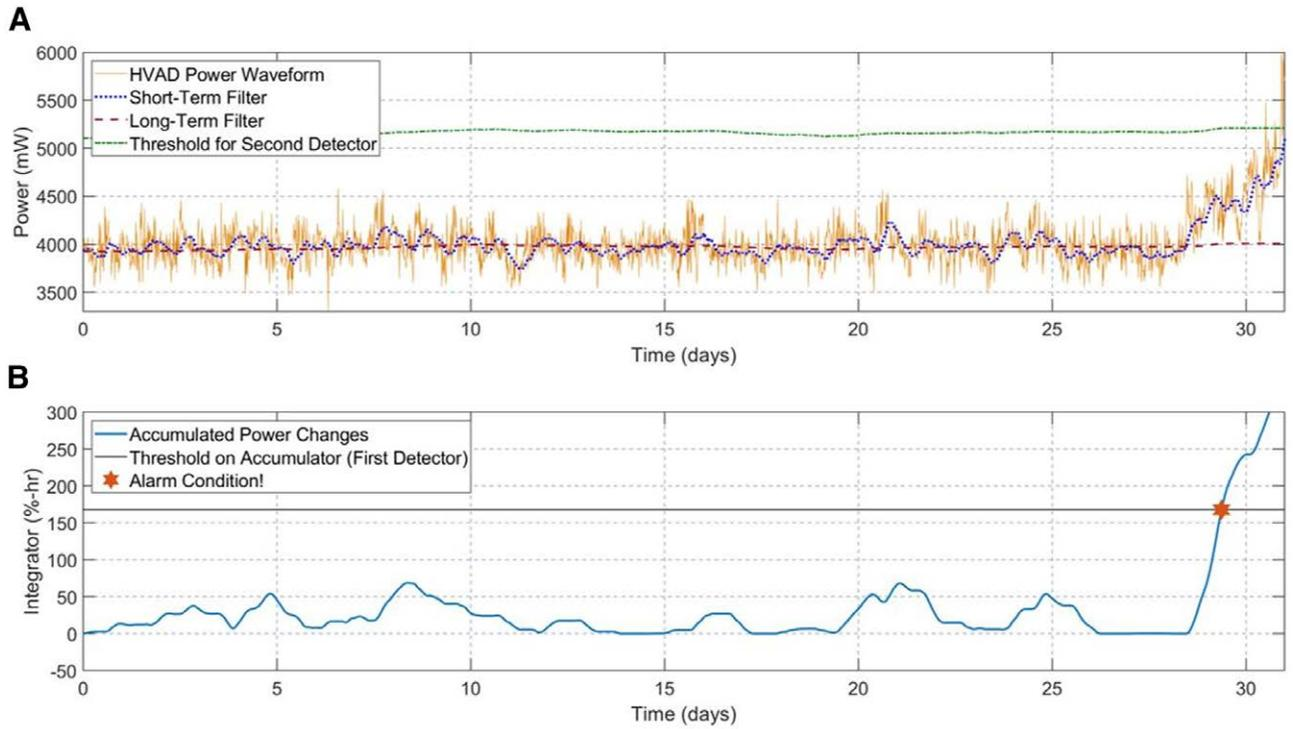
**Figure 2.** Schematic of the power tracking algorithm. **A:** Short-term and long-term filters for the first detector and threshold for the second detector. **B:** Accumulated power changes and threshold for the first detector.
