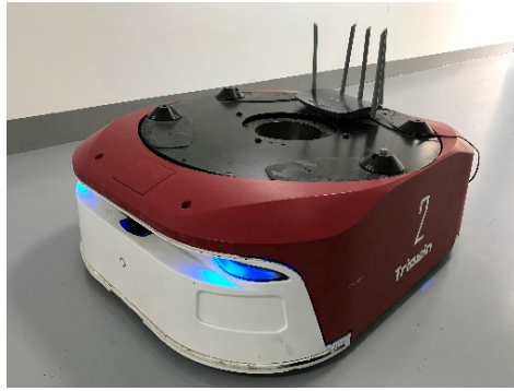
Figure 16. TRIOWIN mobile robot with mounted sensors.
