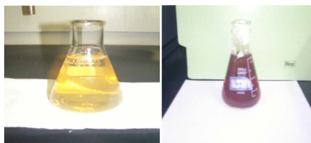
Figure 2 Color change of Rhinacanthus nasutus leaf extract containing silver before (left) and after (right) synthesis of silver nanoparticles.
