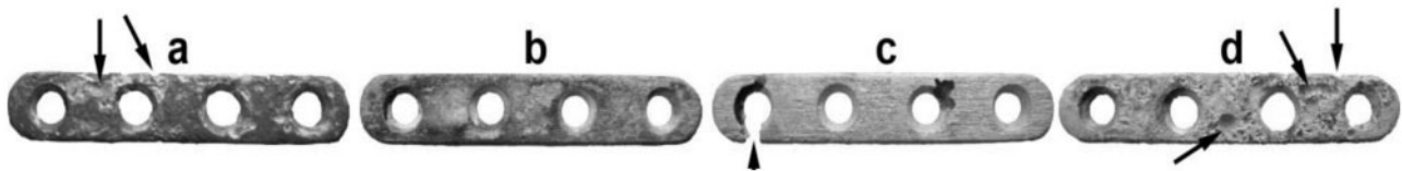
Figure 9. In vivo degradation morphology of bone plates fabricated with (a) JDBM, (b) JDBM covered with brushite coating, (c) AZ31 and (d) WE43, at 18 weeks post-implantation into rabbits
