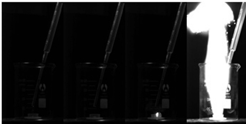
Figure 6. Hypergolic record of compound 8 by high-speed camera (a droplet of 8 into white fuming nitric acid).
