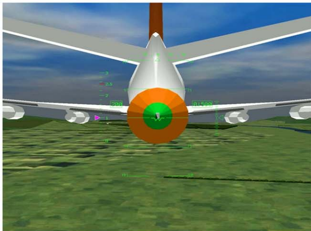
Figure 9. The centre visual display seen by participants (Left) in the HELIFLIGHT simulator (right). Participants were instructed to use the collective lever to control the height of the helicopter, and to keep the W-shaped gull’s wing cross-hair as close as possible to the centre of the refuelling basket. doi:10.1371/journal.pone.0044381.g009
