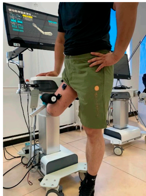
Figure 4. Simulated exercise experiment of the residual limb by the rehabilitation robot.
