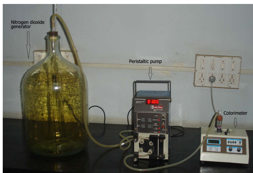
Figure 1. Schematic of laboratory setup used for nitrogen dioxide generation and its measurement using flow type colorimeter.
