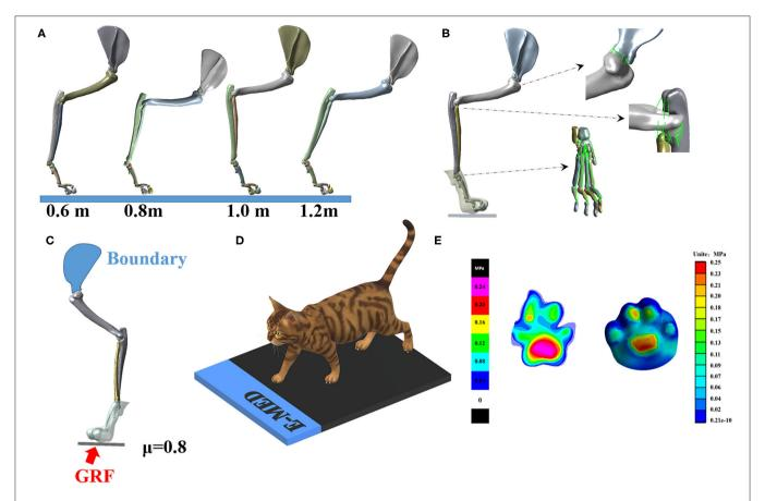
FIGURE 2 | (A) Finite element 3D model of right forelimb at four landing heights. (B) Illustration of ligament and soft tissue of model. (C) Illustration of loading and boundary conditions. (D) Experimental verification of plantar pressure of cat right forelimbs. (E) Experimental verification results (left) and finite element simulation results (right). The scales on the left and right diagrams are different; please refer to their scales.
