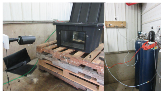
Figure 2. Setup of the gas chamber for Experiment 2. Setup was similar to Experiment 1 except there were two cameras (1) and two acrylic glass observation windows (2). Instead of a ventilator, the vacuum pump created negative pressure and the air it took out was routed through a tube (3) to the outside. The on/off valves (4), tubing, and tanks (5) were similar. However, there was only one tube (6) that went to one mass flow controller and then into the box, instead of two mass flow controllers as was used in experiment 1.
