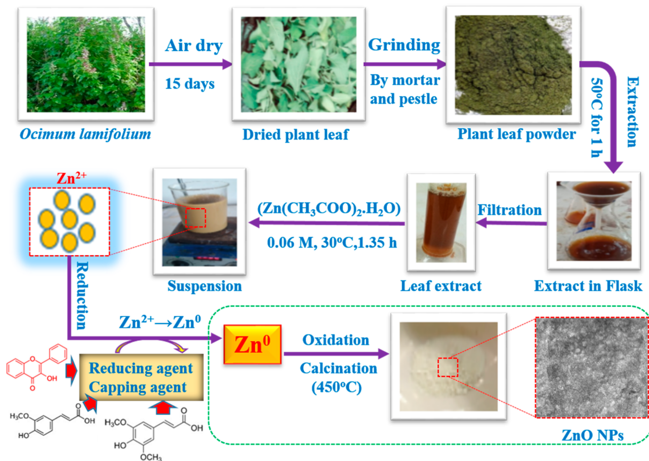
Scheme 1. Schematic Diagram of Green Synthesis Mechanism of ZnO NPs Using O. lamifolium
