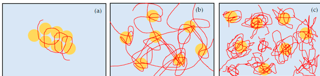
Figure 5. The schematic representation of silica (circle) -PEO (lines) suspension. The states of these figures are: (a) low C_p , (b) Appropriate C_p , (c) too high C_p . When C_p is low, the amount of PEO is not enough to form a gel network. The suspension is cloudy sol. When C_p is appropriate, the number concentration of bridges increases to make bridges among particles. Motion of water is limited in the network, and the suspension turns to gel. If C_p is too high, available adsorption site of silica decreases. PEO is difficult to form bridges between particles, and suspension keeps high viscosity sol.
