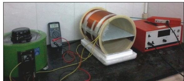
Figure 1: Extremely low-frequency electromagnetic fields generated system contained (from left to right) autotransformer, multimeter, solenoids coils, teslameter and its probe
