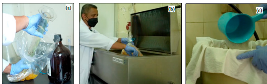
Figure 6. (a). The initial chlorine dioxide addition process is 0.22 KN (kappa number); (b). Heating with a time of 30 min and a temperature of 95 °C; (c). EFB fiber was cooked at 130 °C for 60 min (time to reach maximum temperature was 60 min and held for 90 min).
