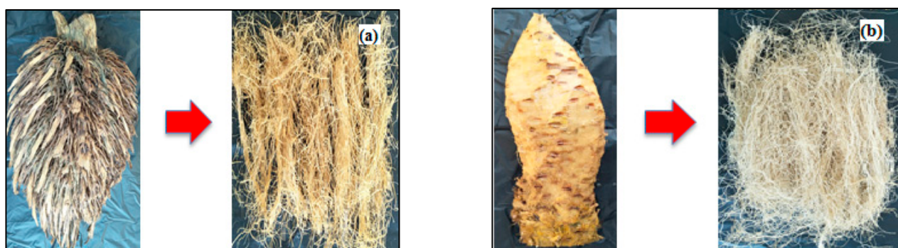
Figure 2. (a). WEFB is converted into fibers with a length of 10–20 cm before the cutting process with a cutting machine; (b). SEFB is converted into fibers with a length of 10–30 cm before the cutting process with a cutting machine.
