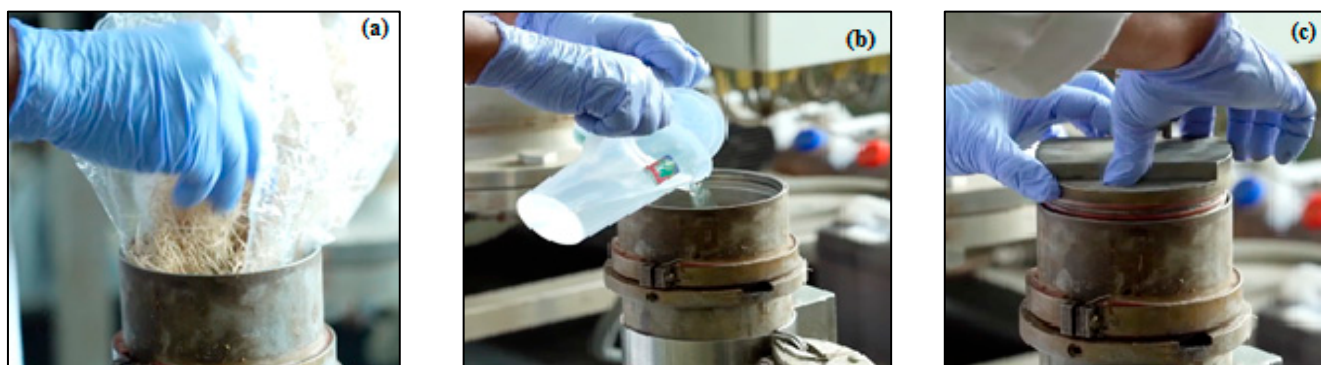
Figure 4. (a). EFB fiber (first sample and second sample) with a length of 2–3 cm and a mass of 300 g was inserted into the rotary digester tube (b). Addition of 1 N sulfuric acid, 0.4% sulfite pre-hydrolysis with a ratio of 1:5 ( w/v ); (c). EFB fiber was cooked at 130 °C for 60 min (time to reach maximum temperature was 60 min and held for 90 min).
