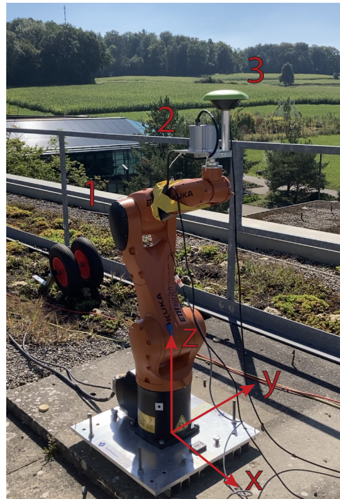
Figure 1. The experiment set-up showing (1) the KR AGILUS-2, KR 6 R900 sixx robot arm, (2) KVH 1750 IMU, and (3) Javad GrAnt G3T Global Navigation Satellite System (GNSS) Antenna. The location of (2) is also where the EpiSensor is placed.
