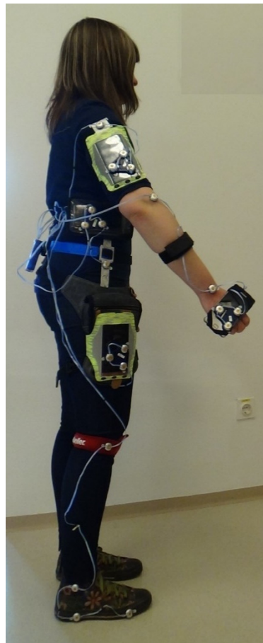
Figure 3. Optotrak's infrared markers attached to anatomical landmarks of the human body and four smartphones.
