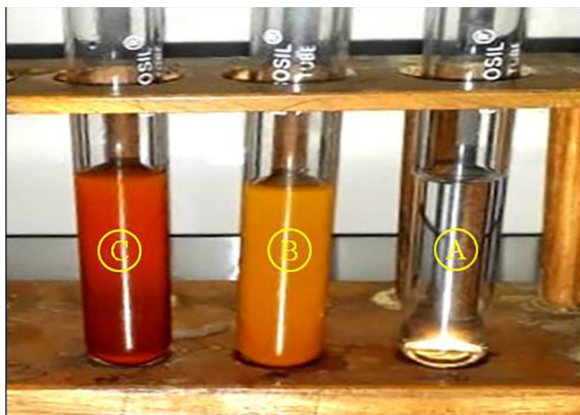
Fig. 5. Visual observations of (A) silver nitrate solution, (B) leaf aqueous extract and (C) synthesized AgNPs.
