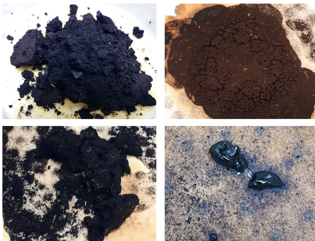
Figure 3. Top left: HC–HTC of SA (0.62 M Fru), 180 °C, 2 h (N/C=0). Top right: HC–HTC of solution SD (0.62 M Fru + 2.92 M urea), 180 °C, 2 h (N/C=0.3). Bottom left: HC produced after hydrothermal carbonization of SM (0.62 M Fru + 0.38 M urea) in acidic conditions (pH value of 1.9), 180 °C, 2 h. Bottom right: Bio-oil produced after hydrothermal treatment of SC (0.62 M Fru + 0.19 M urea) in alkaline conditions (pH value of 9), 180 °C, 2 h.
