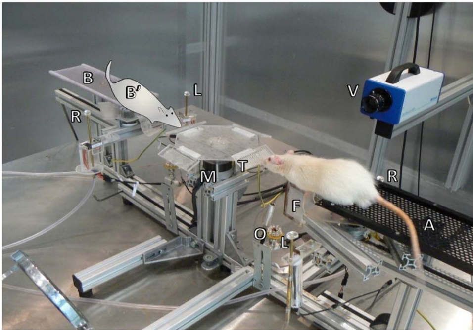
Figure 1. Experimental setup. Photograph of texture palpation taken under visible light. A-platform A, B-platform B, B'-rat position on platform B, M-motor for automated presentation of textures, T-textured plate, F-foot rest, O-optical triggers for touch detection, L, R-left and right water spouts, V-high-speed video camera. While the rat collected the reward, the motor rotated to put one of the four textures, in random order, in position for the next trial. The motorized foot rest (F) was then extended to allow the rat to reach the texture. When the rat withdrew after texture palpation, the foot rest was retracted to prevent the animal from returning to the texture. Optical triggers were positioned in front of the texture to detect touch and the beginning of turn (i.e. the moment when the animal retracted from the texture). The animal's choice was detected by another set of optical triggers (not labeled) located immediately adjacent to the drinking wells. doi:10.1371/journal.pone.0016462.g001
