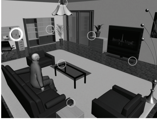
FIGURE 1: The room accommodating the patient. The CRUs and the G-CRU installed across the room are highlighted by the thin circles and the thick circle, respectively. The packet transmitted by the implant is received by multiple CRUs, which then cooperatively make the decision on the implant packet.
