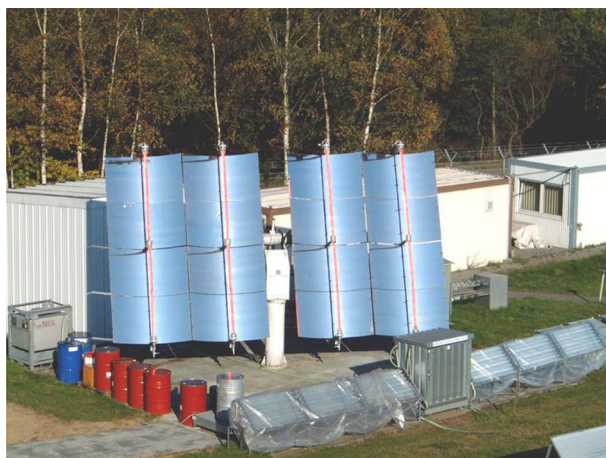
Fig. 6 Photograph of the PROPHIS reactor at the DLR facility in Cologne. The four reaction tubes filled with a red reaction mixture and their parabolic collector are mounted on a Helioman solar tracking system
