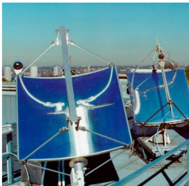
Fig. 9 The line-focusing solar photoreactor at the Max Planck Institute of Mülheim. Reprinted with permission from [38]. Copyright 2016 American Chemical Society
