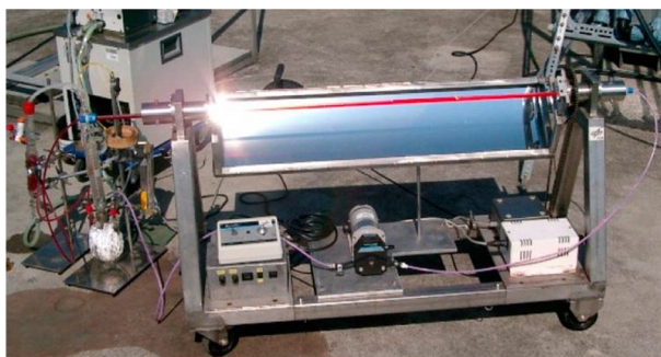
Fig. 11 CPC reactor with holographic mirrors for the solar photooxygenation of 5-hydroxy-1,4-naphthoquinone, sensitized by rose bengal (as evident from the red color of the tube). Reprinted with permission from [38]. Copyright 2016 American Chemical Society
