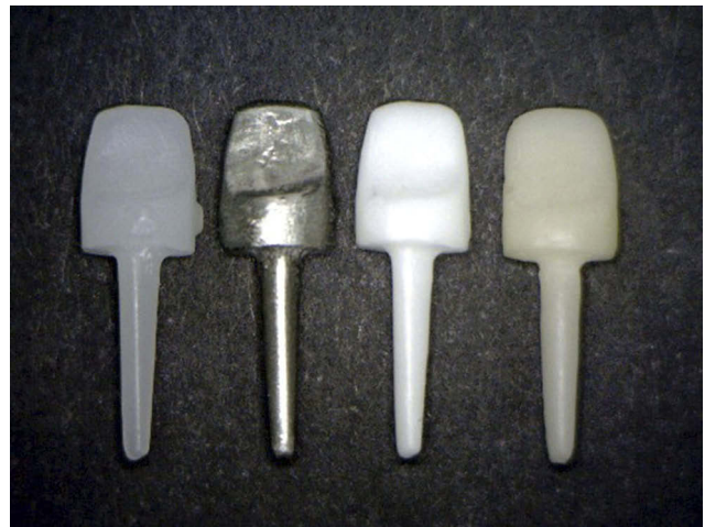
Figure 1 Standardized cast post and core teeth. From the left; CAD/CAM milled wax post and core, cast metal post and core, CAD/CAM milled Zirconia post and core, and CAD/CAM milled PICN post and core.
