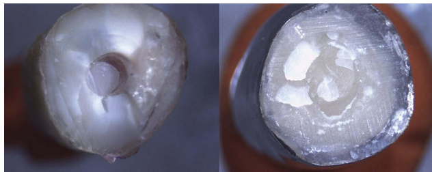
Figure 6 Stereomicroscopic images show a favorable root fracture and post-core fracture in the PICN group.
