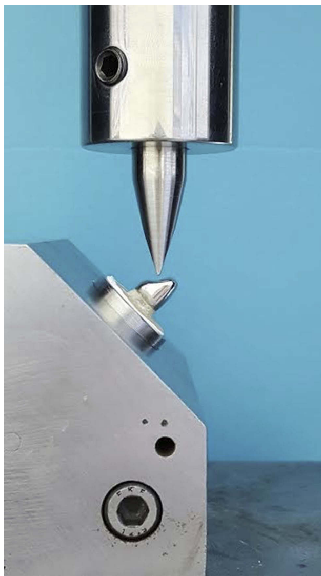
Figure 3 The image shows custom-made assemblies, starting from the superior part; the chisel head is pointed at 135^\circ on the palatal surface of the tested tooth.
