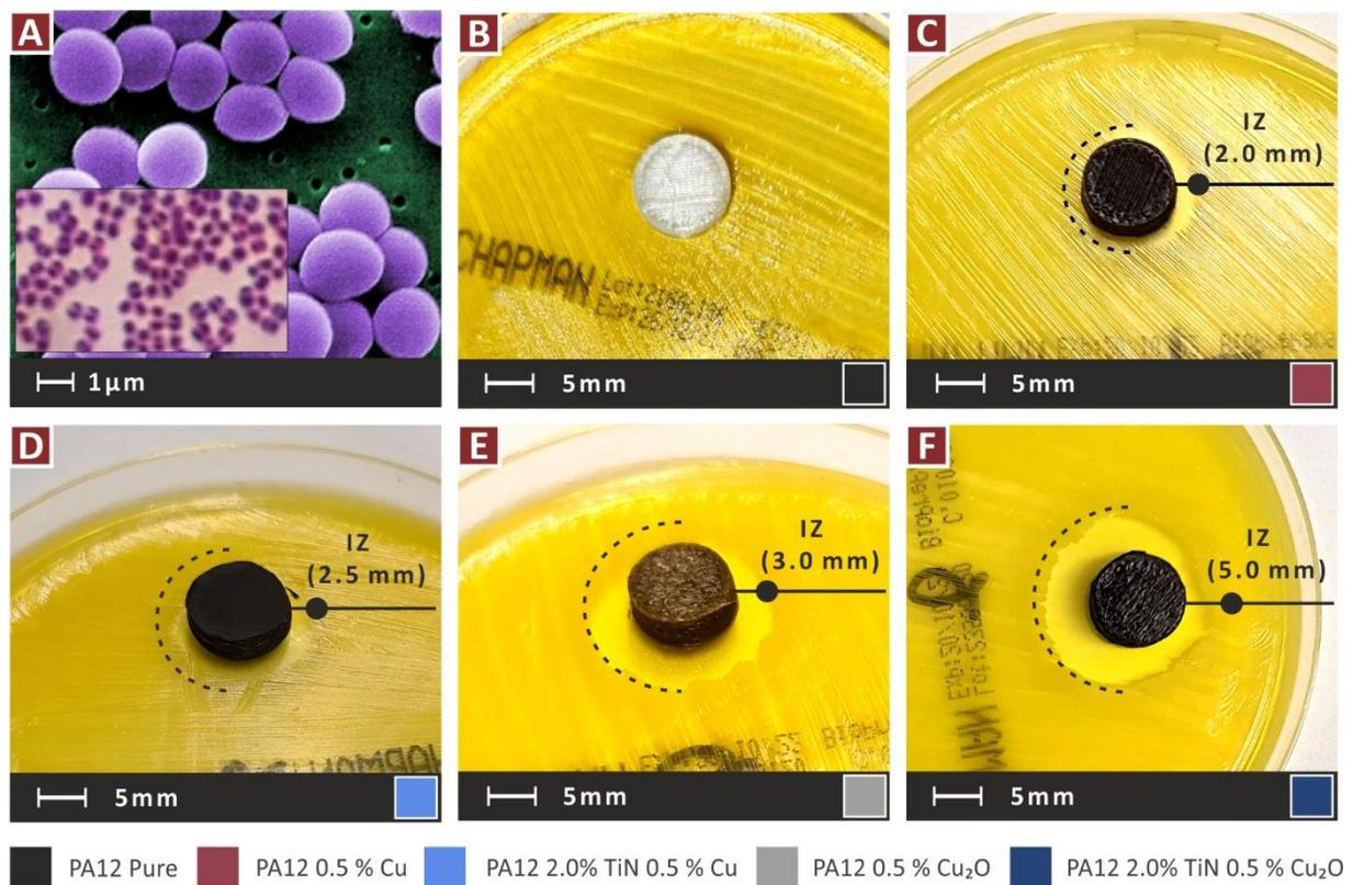
**Figure 17.** *S. aureus* bacterium biocidal performance of the nanocomposites: (A) *S. aureus*, and PA12 (B) pure, (C) 0.5 wt.% Cu, (D) 0.5 wt.% Cu, 2.0 wt.% TiN, (E) 0.5 wt.% Cu<sub>2</sub>O, and (F) 0.5 wt.% Cu<sub>2</sub>O, 2.0 wt.% TiN.
