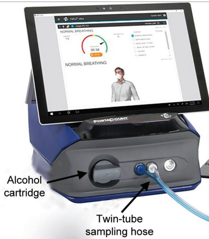
Fig. 3: PortaCount Respiratory Fit Tester 8048 condensation nuclei counter unit. Published with permission from airmet.com.au (Air-Met Scientific Pty Ltd. Nunawading, Victoria 3131, Australia)
