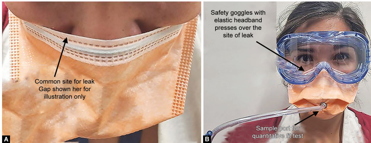
Figs 1A and B: (A) Common site for leaks for N95 respirators; (B) Safety goggles with headband presses the respirator against the skin to seal the gap that results in a leak. The sampling port in the respirator used for QnFT with PortaCount is also shown
