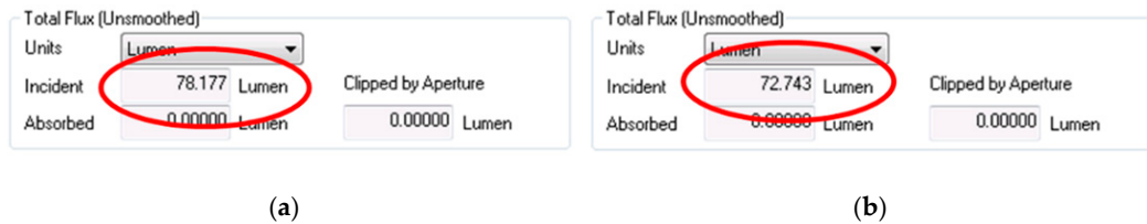
Figure 5. LightTools Light Extraction Efficiency results. (a) results for Silver; (b) results for Aluminum.
