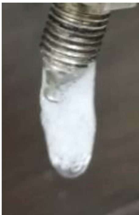
Fig. 13 Snapshot of the CO 2 foam (generated by ODPTA) flowing out at the exit of the sand-pack during the CO 2 -ODPTA solution flooding experiments: high flow resistance at 160 °C generated during flooding process by the Jamin effect of the CO 2 foams, not by the speculative plugging through aggregation or precipitation of surfactant molecules.
