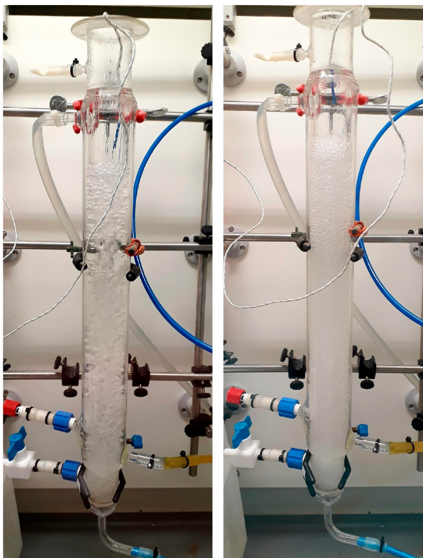
Figure 9. Images of the bubble column operating with (left) pure solvents and (right) dissolved API, operated under same conditions and flow rates.
