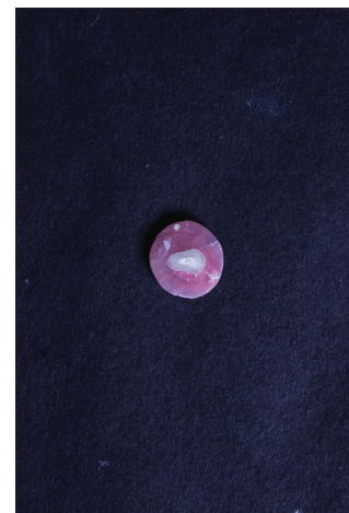
Figure 3: 1.5 mm thick section made using diamond disc
